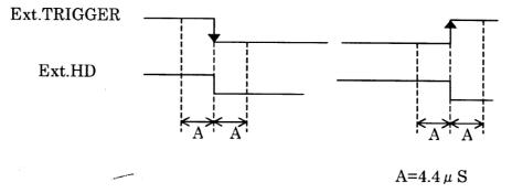
Fig. 7. External trigger and HD relations
